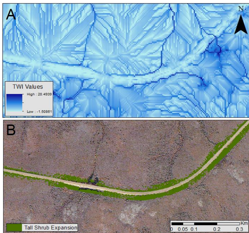
Figure 2-9: Topographic wetness index (A) derived from a LIDAR digital elevation model and a QuickBird satellite image of the same area (B). Darker blue regions on the topographic wetness index represent areas of higher potential wetness. Areas of tall shrub proliferation adjacent to the Dempster are shown as green polygons.
