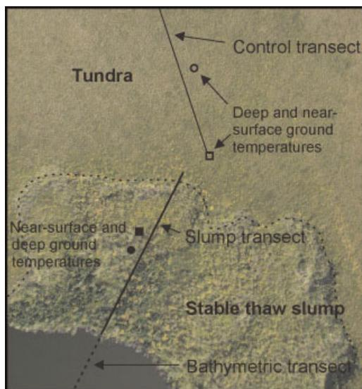
Figure 3 Aerial photograph of site T7 showing locations of transects, near-surface (■□) and deep (○●) ground temperature instrumentation on undisturbed tundra and in a stable thaw slump. The bathymetric transect extending from a disturbed shoreline is also shown. The thin dashed line outlines the scar area.
