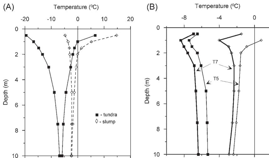
Figure 8 A) Maximum and minimum ground temperature profiles for undisturbed tundra and a stable vegetated slump surface, T7, Richards Island. B) Mean annual ground temperature profiles for undisturbed tundra and stable slump surfaces at T5 near Parsons Lake, and at T7 on Richards Island. Data are for August 2006 to August 2007.
