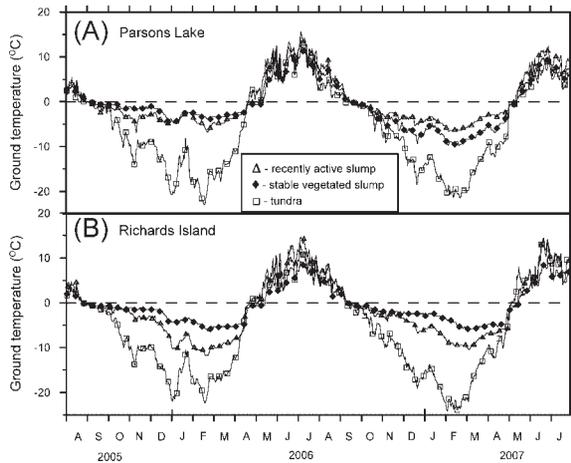
Figure 7 Ground surface temperatures (August 2005 to August 2007) at 5-cm depth for recently active and stable thaw slumps, and undisturbed tundra at A) T5 near Parsons Lake and B) T7 (stable and undisturbed tundra) and T7a (recently active) on Richards Island. The data are daily averages and symbols are plotted at 12-day intervals.
