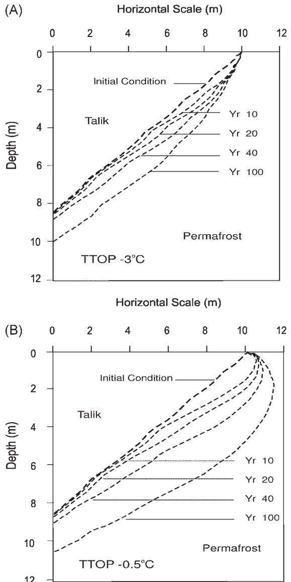
Figure 9 Modelled near-surface talik configuration for a 600-m diameter lake with an adjacent: A) cold (mean annual temperature at the top of permafrost, (TTOP  $-3.0^{\circ}\text{C}$ )); and B) warm (mean annual temperature at the top of permafrost, (TTOP  $-0.5^{\circ}\text{C}$ )) retrogressive thaw slump extending 100 m from the lakeshore. The modelled surface or zero on the vertical scale represents the lake bottom or top of the permafrost.
