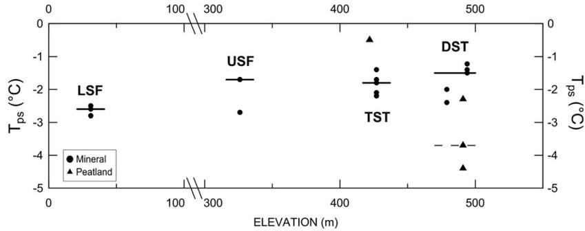
Figure 6 Annual mean temperature near the permafrost surface ( $T_{ps}$ ) across the forest-tundra ecotone for 2010–13. The solid black lines represent the median  $T_{ps}$  from instruments in mineral soil for each vegetation unit, and the dashed line is the median for the DST peatland instrument. See text for abbreviations.
