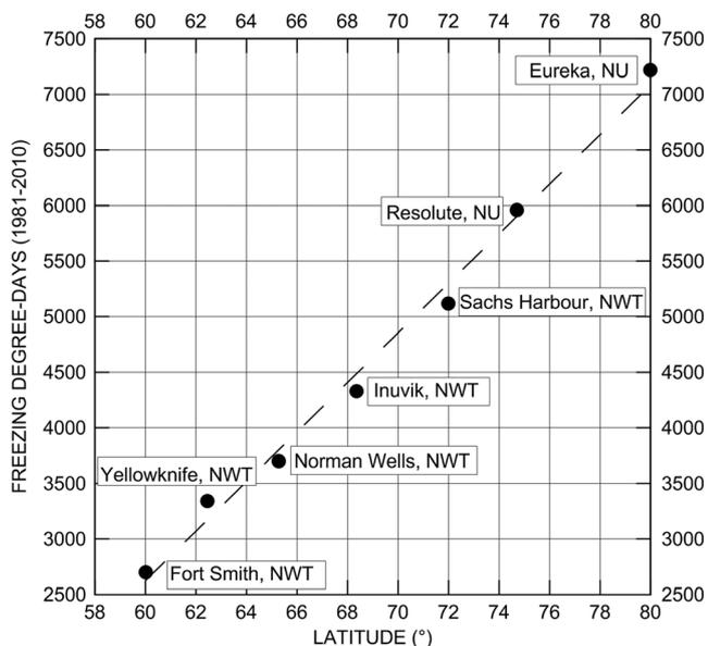
Figure 11 Relation between latitude and average freezing degree days (1981–2010) in seven communities (Environment Canada, 2014). The study area on Peel Plateau is at about 67.2°N, and there were 3968 and 4257 freezing degree days at DST in 2011–12 and 2012–13, respectively. These data are not plotted here, as they are not similar to the long-term averages. See text for abbreviations. NU = Nunavut.
