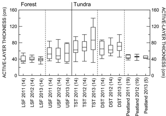
Figure 10 Active layer thicknesses across the forest-tundra ecotone from the four transects in mineral soil and around instrumented sites in peatland (pooled values from the TST and DST peatland). The number of individual points measured is in parentheses. See text for abbreviations.
