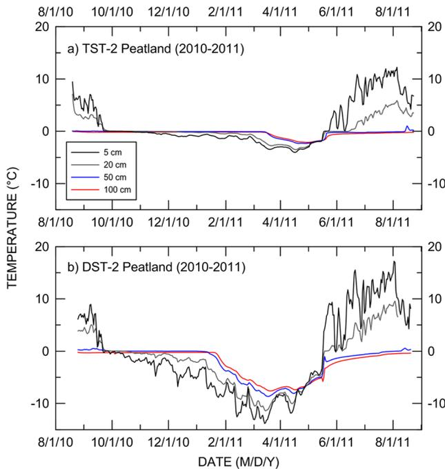
Figure 9 Ground temperatures at (a) peatland at the base of a slope where thick snow accumulates ( $T_s = 1.3\text{ }^\circ\text{C}$ ;  $T_{ps} = -0.5\text{ }^\circ\text{C}$ ), and (b) an exposed peatland where little snow accumulates ( $T_s = -0.8\text{ }^\circ\text{C}$ ;  $T_{ps} = -2.3\text{ }^\circ\text{C}$ ). See text for abbreviations. This figure is available in colour online at [wileyonlinelibrary.com/journal/ppp](http://wileyonlinelibrary.com/journal/ppp)
