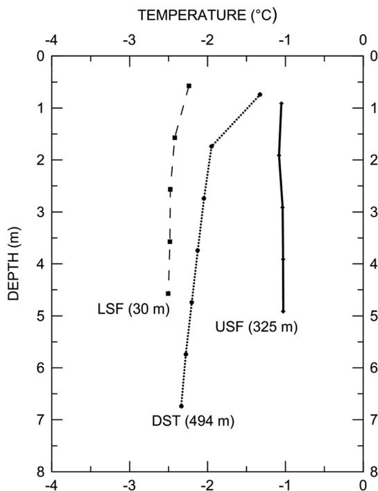
Figure 7 Mean ground temperatures for September 2012 to August 2014. The symbols on each line represent the thermistor locations. See text for abbreviations.
